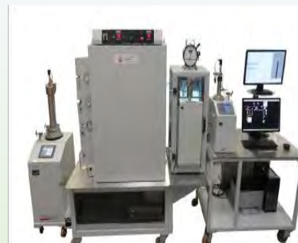
Newly installed Slim Tube apparatus for MMP determination
