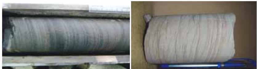
Core with laminated sedimentary structures
