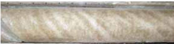
C : Fractured shale within a massive, light grey sandstone
