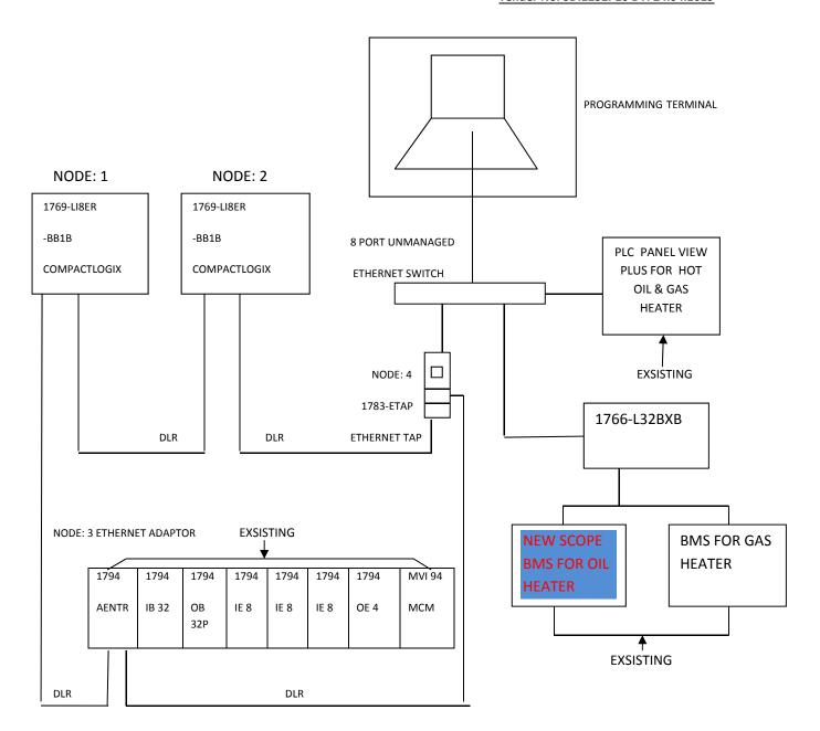
DEVICE LEVEL RING- ETHERNET CABLE
