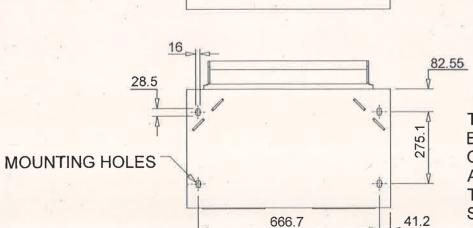
THE FILL STATION UNIT MUST BE ANCHORED TO THE FLOOR OR OTHER STABLE STRUCTURE AND IF POSSIBLE, BOLTED TO A WALL USING STANDOFFS / EXTENDERS
