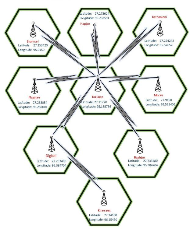
Both the link are running at 2.4GHz and 5.8Ghz frequency band.
