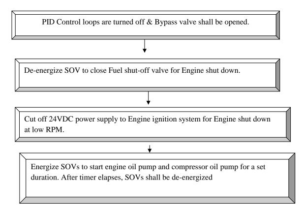
In any of emergency stop, LCP shall generate Closing command to Fuel shut-off valve SOV & Cut off 24VDC power supply ignition system at same time.
