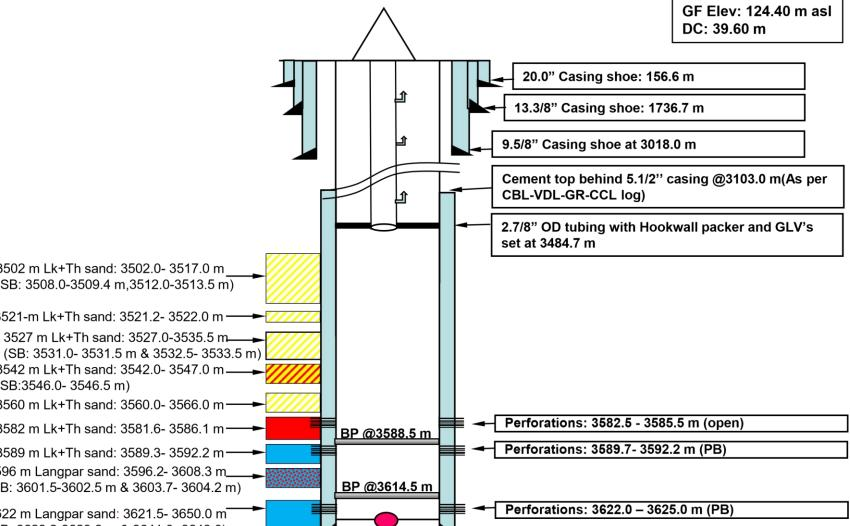
5.1/2" Float Collar/ Casing Shoe = 3641.2 / 3653.6 m (20 lbs/ft, P-110XBTC, N-80XBTC)
